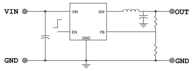
Note: When using a solid or ceramic input Cap, It is recommended to parallel a TVS diode.
